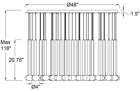
Fixtures weighing 35lbs. or more must be supported and installed independantly of the ceiling outlet (junction) box and require additional support in the ceiling where the fixture is being installed.
